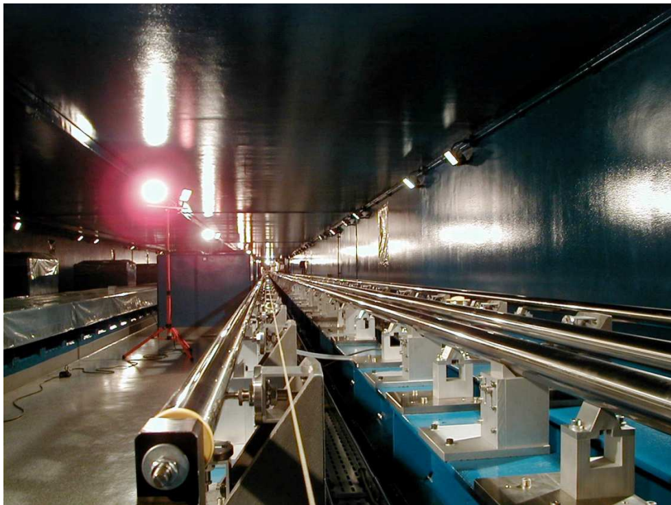
A view along the Interferometric Tunnel, with the rails for two of the VLTI Delay Lines. Courtesy of ESO.
