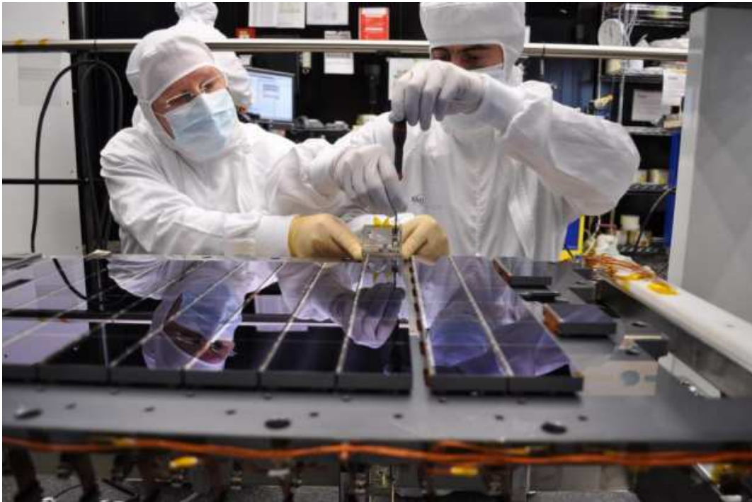
Integration of the hugely successful European e2v Technologies CCDs onto the support structure for the focal plane of the Gaia satellite at Astrium in Toulouse. Image courtesy of Astrium.
