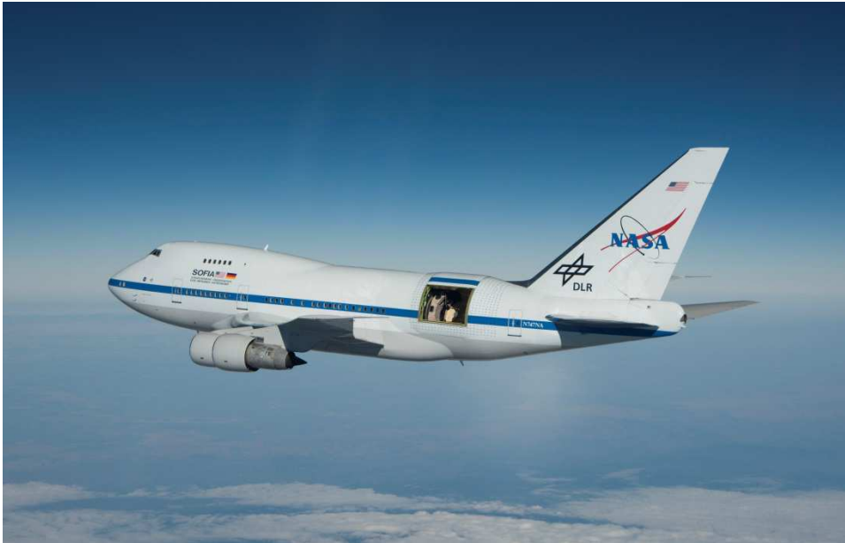
The SOFIA airborne observatory housing a German-built 2.5m telescope. Photo courtesy of Jim Ross/NASA.
